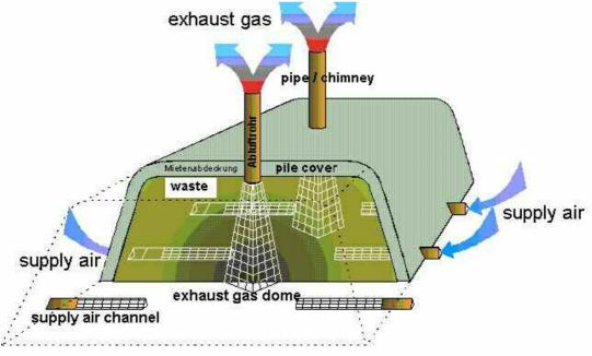
Figure 1 Dome aeration windrow (modified from Brummack et al., 2004)
