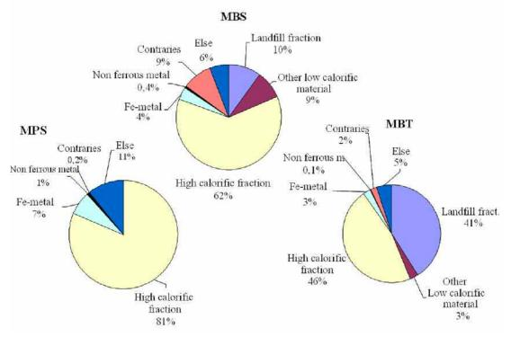
Figure 3-2 Fractioning of output flow with regard to total output (without loss due to degradation and drying) of the different plant concepts
