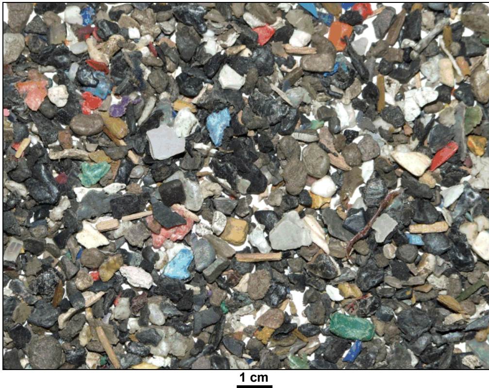
Figure 2 Example of different materials constituting the plastic waste product after the shredding phase of light fractions resulting from car dismantling.
