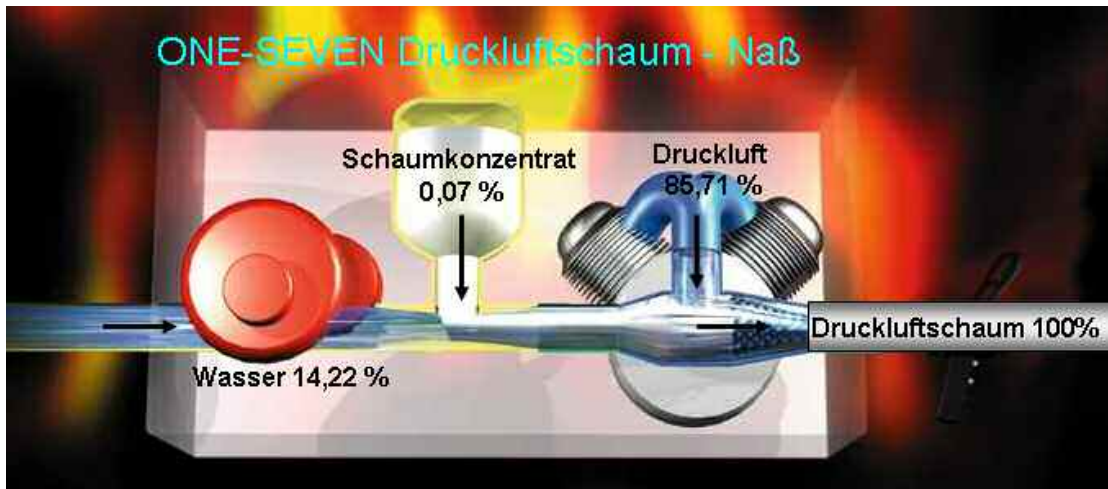
Figure 4: Compressed air foam ONE SEVEN (wet): Water 14.22%; Foam concentrate 0.07%; Compressed air 85.71%; Compressed air foam 100%
